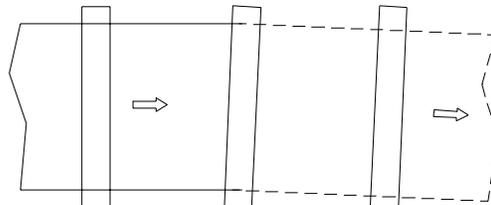
**NEVER USE THE DRIVE OR TAIL SHAFTS (END ROLLS) TO TRACK THE BELT.** This can cause the belt to stretch on one side leading to permanent tracking problems.
