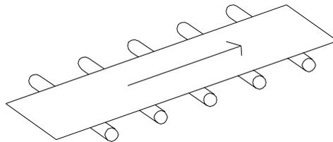
**ROLLER SUPPORT SPACING:** On the loaded side, rollers should be spaced close enough together to fully support the belt and the load being carried with little or no belt sag between rollers.
