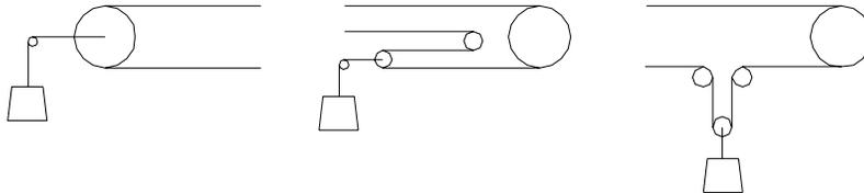
**MECHANICAL TAKE-UP:** A pneumatic or hydraulically actuated cylinder can also be used to provide an automatic take-up system. Designs for this style would be similar to the counter-weight take-up, replacing gravity with the mechanical power of a cylinder. The benefits of a mechanical system are that it is easier to adjust than the counter-weight system, and doesn't require the vertical space. Care should be taken to insure the take-up doesn't tension the belt.
